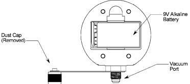
Rear View (Battery Cover Removed)
