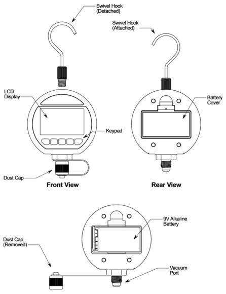
**Rear View (Battery Cover Removed)**
