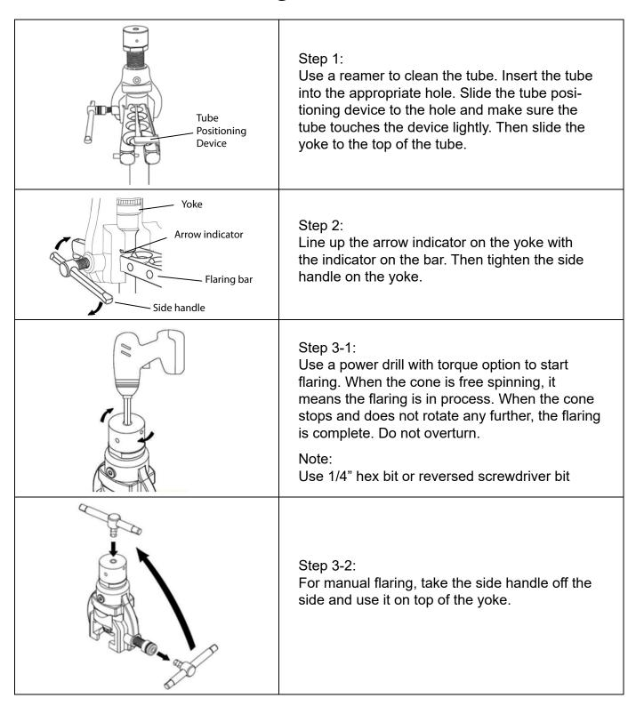
Note: After some uses, clean the debris off the eccentric cone to ensure the smoothness of the cone. Also, for a longer lifespan, use lubricant at the thread to prevent rust.
