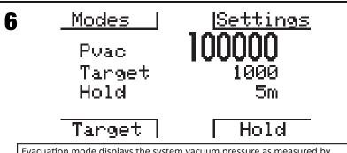
While on any modes screen, tap on any of the four buttons next to the screen once to bring up the button webbing; the button webbing will
