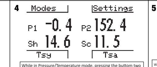
While in Pressure/Temperature mode, pressing the buttom two buttons will alternate between various temperatures. System superheat and subcooling shown.
