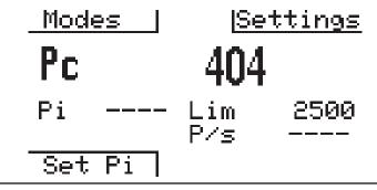
Once you are ready to begin the pressure hold test, bring up the button webbing then press "Set Pi". This will set the current vacuum pressure as the initial system pressure and begin monitoring for a rise in vacuum pressure.
