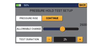
Allowable change is the maximum allowable vacuum pressure the system is allowed to reach before failure. Set the allowable change value by adjusting the slider bar. Adjust the duration of the pressure hold test by tapping the "+" and "-" buttons. When ready to begin the pressure rise test, tap the Continue button next to Pressure Rise.
