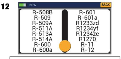
The refrigerant menu allows you quick select a desired refrigerant. Drag the slider bar to the correct page and tap the refrigerant to select it.
