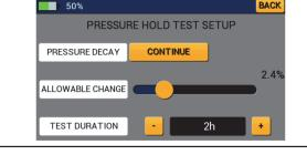
The Pressure Hold mode displays the change in pressure of the system during a standing pressure test. Allowable change is the percentage of the current system pressure the system is allowed to drop before the pressure test is deemed a failure. Set the allowable change percentage by adjusting the slider bar. Adjust the duration of the pressure Decay test by tapping the "+" and "-" buttons. Tap the Continue button next to Pressure Decay to begin the pressure hold test.
