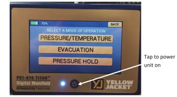
Power the unit on by pressing the power button once. Select the desired mode of operation from the modes menu.
