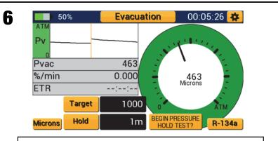
Once the Vacuum Hold timer has depleted, the user is prompted to start a pressure hold test. Tap the button to advance to the pressure hold setup screen.
