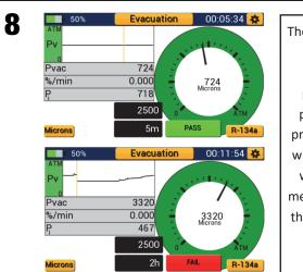
The Pressure Rise test will monitor the current vacuum pressure and the percent change in pressure. The device will prompt the user with a Pass or Fail message depending if the system passes or fails the test respectively.
