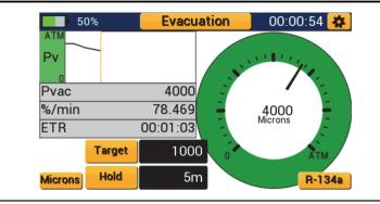
Evacuation Mode displays vacuum pressure as measured by a YJ auxiliary vacuum sensor. Plug the vacuum sensor into either A1 or A2 on the back of the device. Tap Target to set the target evacuation pressure. Tap Hold to set the duration of the vacuum hold timer.
