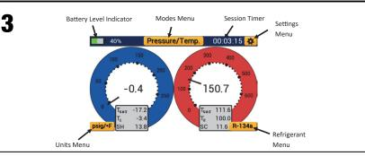
Pressure/Temperature Mode displays system pressure, temperature, saturation temperature, system superheat and subcooling. Settings can be accessed by tapping the settings icon in the upper right corner. The modes menu can be accessed by tapping the button labeled with the name of the current mode at the top of the screen. The units and refrigeration menus can be quickly accessed by tapping the buttons in the lower left and right corners respectively.
