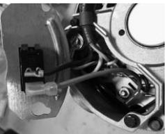
4. Reattach the rocker switch plate to the motor body and tighten the (2) screws.
