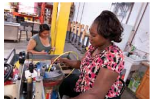
Yellow Jacket hoses are cut and proper fittings are applied to each end at the Bloomington, Minn. production facility.
