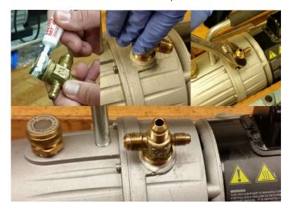
NOTE: NPT should neve be unthreaded to meet orientation. Only tighten. Loosening could compromise thread seal
