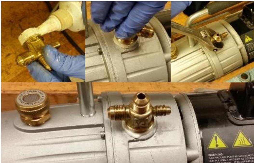
**NOTE:** NPT should never be unthreaded to meet orientation. Only tighten. Loosening could compromise thread seal
