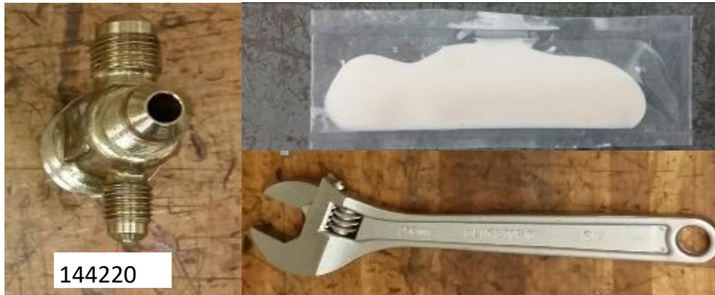
Cut corner off Loctite packet to make dispensing spout.
