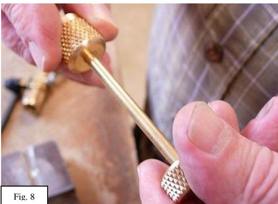
A-8. Place the “pre-assembled nut” onto the shaft. Be sure the open end of the “nut” faces out when installing.
