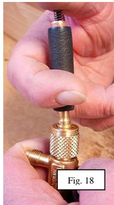
B2. Place the “gasket” into the tool shown. Install the gasket into the end of the “ball valve” closest to the “side port” (of the ball valve).
