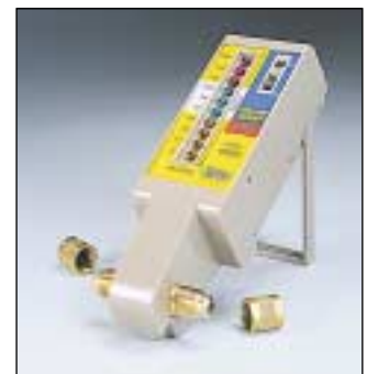
Constant current or voltage is applied to thermistor-style electronic vacuum gauges, like the one pictured above, while evacuating refrigerant.
