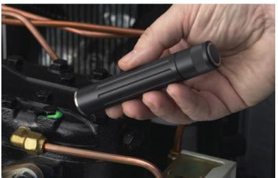
Whether the system runs continuously or part-time, the dye solution in the Yellow Jacket Micro LED UV Leak Detection Kit is ready in the system 24 hours a day to help find even the smallest leaks with the lightweight Micro LED UV lamp, said manufacturer Ritchie Engineering.
