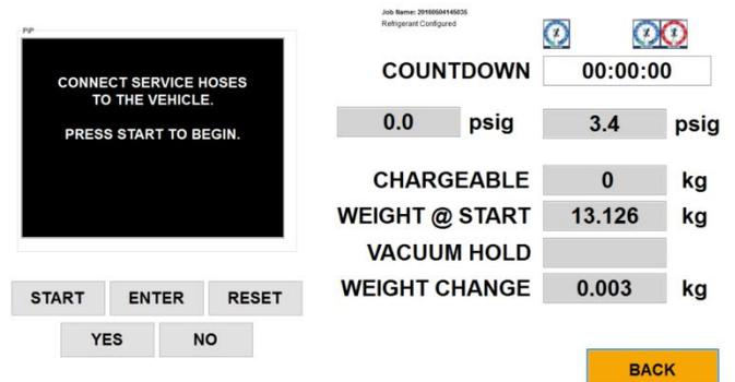
10. During the recovery operation, refrigerant is removed from both the high and low side of the automobile air conditioning system. The tablet will display the amount of refrigerant currently recovered during the cycle and the
