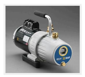
Wide mouth oil reservoir port for easier, cleaner filling. The YELLOW JACKET® BULLET™ vacuum pump is a two-stage rotary vane oil-sealed 7 CFM pump that pulls down to 25 microns or better.
