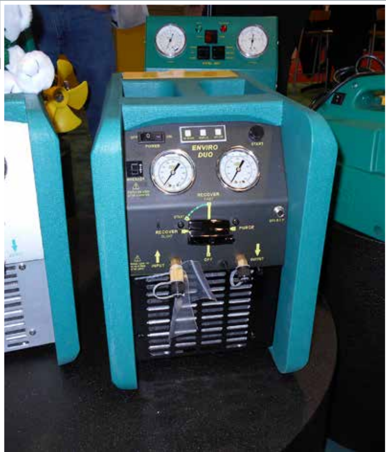
REFCO ENVIRO-DUO: The Refco Enviro-Duo is approved for use with class A2 mildly flammable refrigerants, including R-32, -1234yf, and -1234ze.
