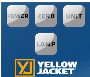
“LAMP”: Press to light the backlight and it will last for 10s. Press and hold for 3s to keep the backlight on all the time, buzzer will beep once as indication. Press again to turn off the backlight.
