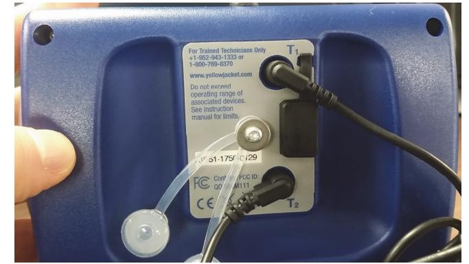
Connect the low side temperature probe to T1 on the back of the device. Connect the high side temperature probe to T2 on the back of the device.
