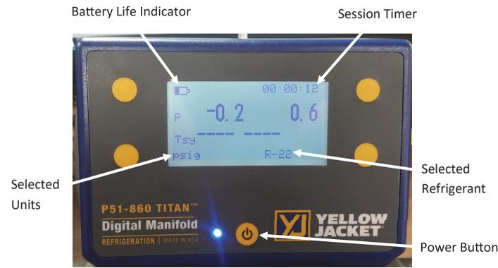
Power the unit on by pressing the power button once. The unit automatically defaults to Pressure/Temperature mode. This mode displays system pressure and temperature as measured by two auxiliary YJ temp probes.
