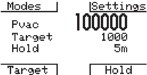
Evacuation mode displays the system vacuum pressure as measured by an auxiliary YJ vacuum probe (P/N 67030). Plug the YJ vacuum probe into either a T1 or T2 on the back side of the device. Tap any button to bring up the button webbing. Press Target to set the Target Evacuation pressure. Press Hold to set the duration of the Vacuum Hold Timer. Once Target Evacuation pressure and Hold Timer have been set, begin the evacuation.
