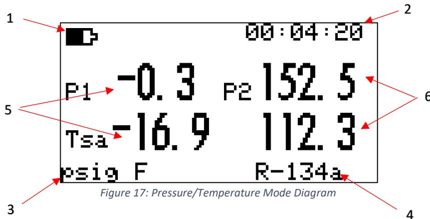
Figure 17: Pressure/Temperature Mode Diagram
