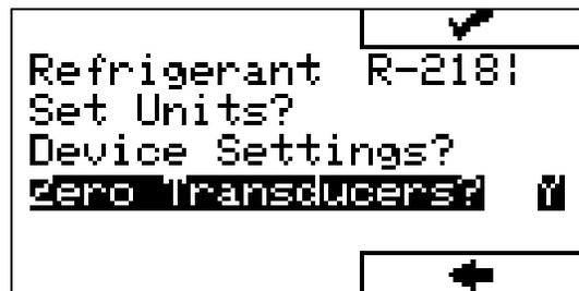
Figure 34: Confirming the Zeroing Selection
