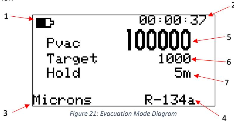
Figure 21: Evacuation Mode Diagram
