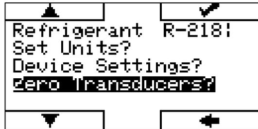
Figure 33: Zeroing the Pressure Transducers
