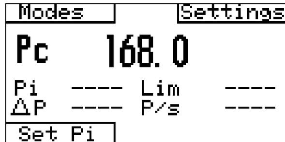
Figure 27: Pressure Hold Test - Setting Initial Pressure
