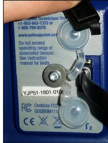
Figure 14: Connecting to the Micro-USB
