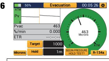
Once the Vacuum Hold timer has depleted, the user is prompted to start a pressure hold test. Tap the button to advance to the pressure hold setup screen.
