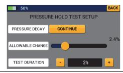
The Pressure Hold mode displays the change in pressure of the system during a standing pressure test. Allowable change is the percentage of the current system pressure the system is allowed to drop before the pressure test is deemed a failure. Set the allowable change percentage by adjusting the slider bar. Adjust the duration of the pressure Decay test by tapping the "+" and "-" buttons. Tap the Continue button next to Pressure Decay to begin the pressure hold test.
