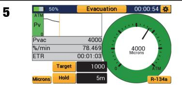
Evacuation Mode displays vacuum pressure as measured by a YJ auxiliary vacuum sensor. Plug the vacuum sensor into either A1 or A2 on the back of the device. Tap Target to set the target evacuation pressure. Tap Hold to set the duration of the vacuum hold timer.
