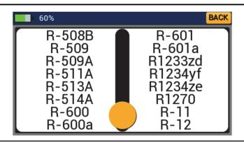
The refrigerant menu allows you quickly select a desired refrigerant. Drag the slider bar to the correct page and tap the refrigerant to select it.
