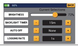
The device settings menu allows the user to adjust the display brightness, backlight dimer timer, device auto off timer, and data logging sampling rate. Use the slider bar to adjust the percentage of backlight brightness. Tap the "+" and "-" buttons to adjust the remaining device settings. Tapping the back button will save the current selections and return to the settings menu.
