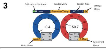
Pressure/Temperature Mode displays system pressure, temperature, saturation temperature, system superheat and subcooling. Settings can be accessed by tapping the settings icon in the upper right corner. The modes menu can be accessed by tapping the button labeled with the name of the current mode at the top of the screen. The units and refrigeration menus can be quickly accessed by tapping the buttons in the lower left and right corners respectively.
