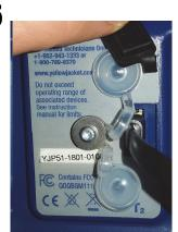
ACCESSING DATA LOG FILES- Connect the unit to a PC via the provided USB to micro-USB cable and power the unit on. The P51-870 will open as a removable drive. Data logs can be copied to the PC for editing and storage. To disconnect the device, eject it as you would a removable flash drive.
