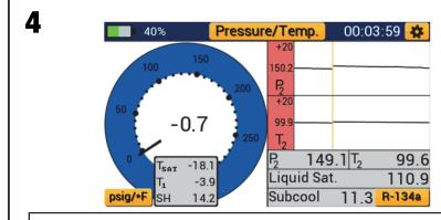
While in Pressure/Temperature mode, tapping the center of either gauge will convert the gauge into a graph. Tap the center of the graph to convert the graph back to a gauge.
