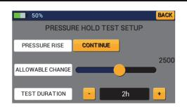
Allowable change is the maximum allowable vacuum pressure the system is allowed to reach before failure. Set the allowable change value by adjusting the slider bar. Adjust the duration of the pressure hold test by tapping the "+" and "-" buttons. When ready to begin the pressure rise test, tap the Continue button next to Pressure Rise.
