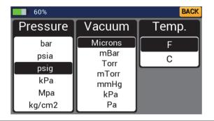
The units menu allows the user to quickly select a unit of measure for pressure, vacuum, and temperature. Tap any unit in the menu to select it. Tapping the back button will exit the units menu and save current selections.
