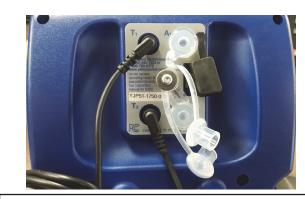
Plug the low side temperature probe into T1 on the back of the device. Plug the high side temperature probe into T2 on the back of the device.
