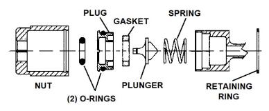
cause the plunger to actuate the valve core before a good seal is formed. To improve the consistency of the SealRight's ability to prevent blow back, the plug has been redesigned and this gasket has been shifted to
