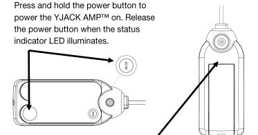
Note the Bluetooth® ID on the back of the device, this ID will be used to assign the device readings in the YJACK VIEW™app or on the P51-870 TITAN® Digital Manifold.
