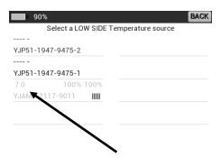
The current readings will display above the YJACK AMP™ Bluetooth® ID. The readings will update every second and be stored to the P51-870's internal data log.
