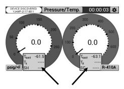
Tap either of the gray temperature boxes at the bottom of the screen to access the probe assignment screen.
