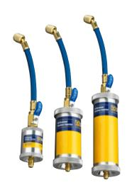
Body and cap are rugged aluminum with an "O" ring seal. 1/4" Male fitting at one end with Schrader. A ball valve for control on other end with a short length of hose. Valve depressor in 1/4" Female end. 600 psi working pressure.
