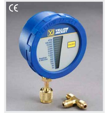
The digital LCD economy vacuum gauge indicates air and moisture have been removed from the system. Track down the 14 level bargraph from atmosphere to 25 microns to know that the system is clean and the vacuum pump is performing properly. Packaged complete with 9V alkaline battery and hanging hook.
