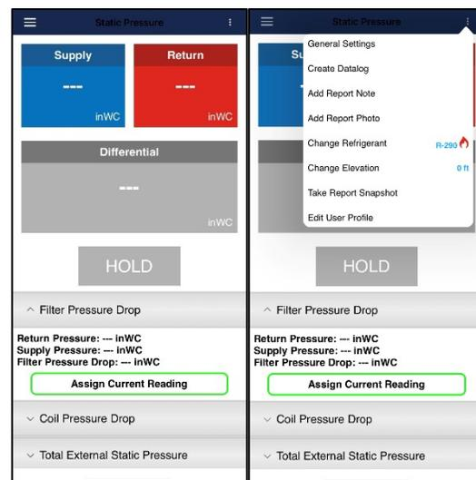
levels will be displayed. Pressures will be displayed as a large digital number to show measurement changes over time. If the system is initially at balanced pressure, the reading is displayed as 0 inWC (or other unit equivalent) until the system pressure differentials change from that level. From the Static pressure reading screen, a Filter Pressure Drop, Coil Pressure drop,
