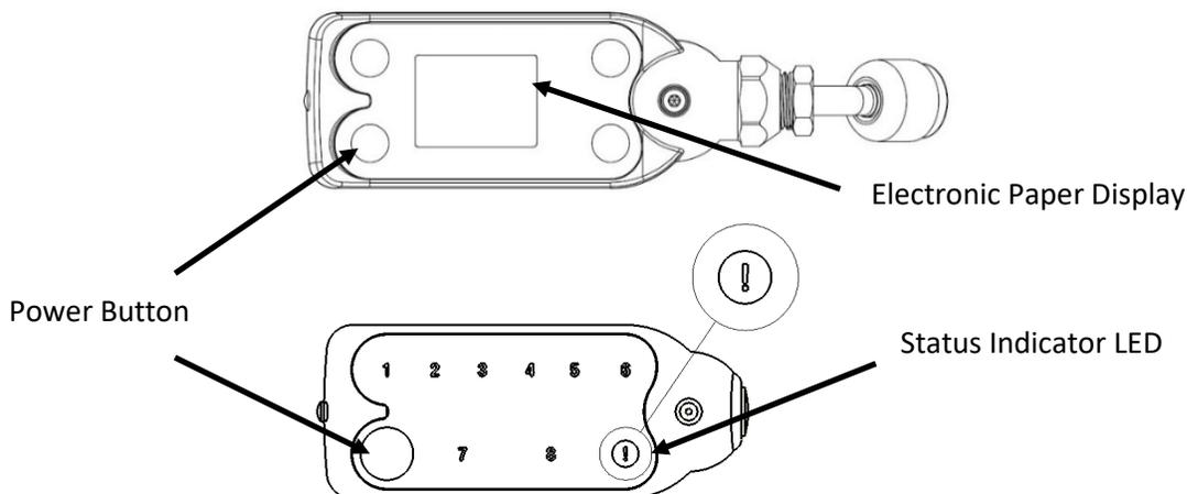
When using the YJACK PATH®, numeric LEDs 1-8 will illuminate to indicate the number of YJACK® and P51-870 TITAN® devices within range.
