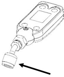
Remove the red plug from the brass quick coupler nut. Then the device can be attached directly to the side port of a core removal tool or to a system service port. A 5/16" adapter (19121 straight or 19221 90 degree) can be used for systems with 5/16" connections. For the most accurate system vacuum readings and to avoid contamination of the sensor, it is not recommended to connect the vacuum gauge directly to the vacuum pump.
