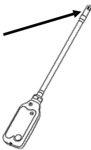
Remove the black vinyl cap covering the sensing element. Form the flexible wand to the desired shape and place the sensing element within the ventilation system or wherever psychrometric data is desired. If there is a ferrous metal surface near the placement of the Dew, the magnet on the bottom of the radio module can be attached to the surface for a more secure connection.
