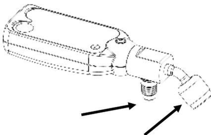
Remove the red plug from the brass quick coupler nut. Make sure the pressure transducer has been zeroed (this will be covered in more detail later) and attach the device directly to the system low-side or high-side service port. A 5/16" adapter (19121 straight or 19221 90 degree) can be used for systems with 5/16" connections. The integrated charging port on the back of the device can be connected to a charging hose for adjustment of system charge while continuing to monitor system pressure.
