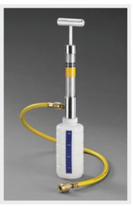
Self-contained injection system for inducing up to 16 oz. of universal AC/R dye into the largest systems. Add to the lo-side. Easily works on all system pressures to 300 psi, .35 oz. per stroke. Hose included with SealRight end.
