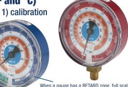
When a gauge has a RETARD zone, full scale is considered to be the last marked reading prior to entering the RETARD zone. For example, this gauge has a full scale reading of 120 psi. Gauge accuracy is not specified in the RETARD zone.
