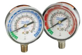
Ammonia gauges are designed for use on manifolds and as permanent gauges on any system or equipment charged with ammonia. The Bourdon tube is made of 316 stainless. The dials show dual temperature and pressure scales. All gauges are equipped with restrictors to protect the gauges against pulsating pressure.
