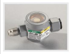
Use with YELLOW JACKET® RecoverX and RecoverXLT machines. Indicates when all liquid has been recovered so you can switch immediately to vapor cycle and speed up the recovery process. 1/4" flare x 1/4" female flare.
