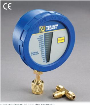
The digital LCD economy vacuum gauge indicates air and moisture have been removed from the system. Track down the 14 level bargraph from atmosphere to 25 microns to know that the system is clean and the vacuum pump is performing properly. Packaged complete with 9V alkaline battery and hanging hook.
