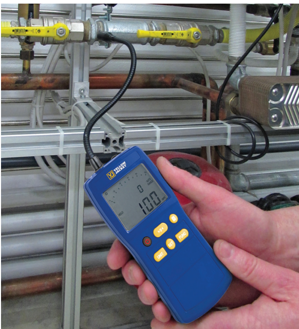
Displays Readings in PPM, % Vol. and % LEL
