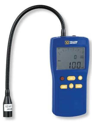
Displays Readings in PPM, % Vol. and % LEL
