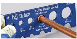
Set the flared tubing into the proper gauge hole where there is a stop midway through for proper diameters. An undersized diameter will pass through and an oversized flare will not fit at all.
