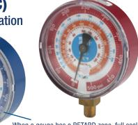
When a gauge has a RETARD zone, full scale is considered to be the last marked reading prior to entering the RETARD zone. For example, this gauge has a full scale reading of 120 psi. Gauge accuracy is not specified in the RETARD zone.
