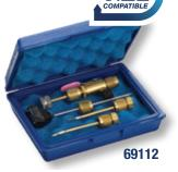
Once charging is complete, use the RealTorque® Core Removal tool to properly tighten the system Schrader core to the manufacturer's recommended torque value of 3-5 in-lb with its integrated torque mechanism. The kits also include all the tools necessary to replace Schrader cores without losing system pressure even if the core or mating core threads are damaged. Kits are available for 1/4" (69111) and 5/16" (69112) systems.
