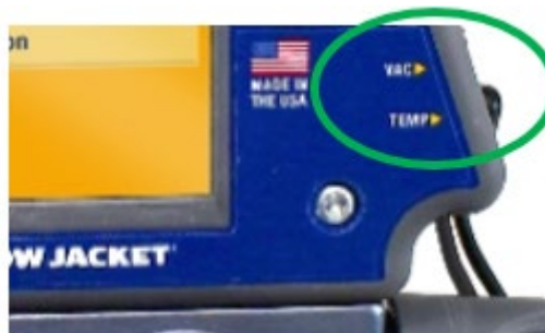
Figure 10: Connecting the Vacuum Sensor
