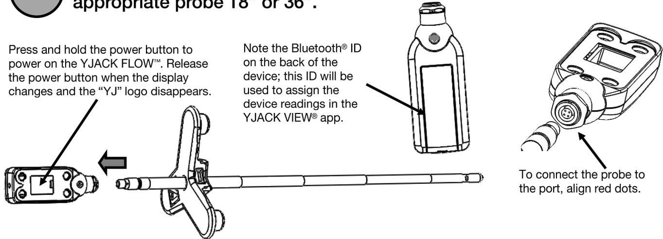
To connect the probe to the port, align red dots.
