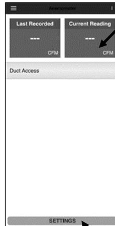
Tap in the reading display area to assign the YJACK FLOW™ device
