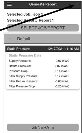
Tap on "SETTINGS" to enter into round or rectangular duct, as well as straight line or AHRI standard multiple point data collection for recording all point average inside of ducts
