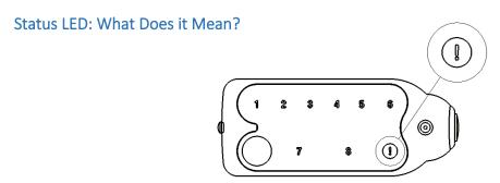
When powering on the YJACK® device, hold the power button until the status LED illuminates solid yellow, then release the power button. Once powered on, the LED will flash every time the YJACK® devices readings are broadcast, every 2 seconds. When the battery level reaches 10%, the LED will flash red to indicate the low battery condition. When powering off the device, the LED stays red until the power button is released and the device is powered down.
