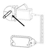
Depress the clamp lever and place the CT around the hot or neutral wire where AC current is to be measured. Make sure the clamp jaws are fully closed for best accuracy. If there is a ferrous metal surface near the placement of the clamp, the magnet on the bottom of the radio module can be attached to the surface for a more secure connection.
