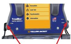
Plug the low side temperature probe into T1 on the lower left side of the device.
