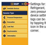
Refrigerant, units, zero pressure sensors, device settings and logs can be accessed by tapping the settings icon in the upper right corner.
