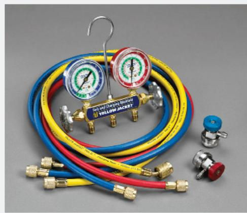
Forged body is solid brass for durability. Full porting maximizes capacity. Metal valve handles are full size for easy operation. Hose anchors are forged into back of body at 45°. Flutterless™ technology helps minimize needle pulsation for easier, more accurate readings. Double “O” ring piston for reliability and long service life. 🇺🇸
