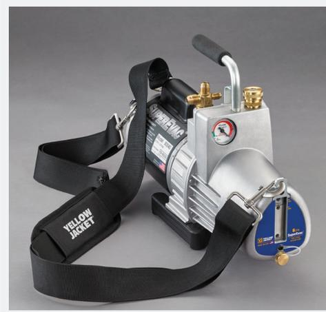
The SUPEREVAC® vacuum pump is a highly efficient, two-stage rotary vane oil-sealed pump field-rated at 15 microns or better. The lower the micron rating, the better the pump performance.
