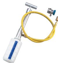
Oil recharge pump for replacing oil in auto A/C systems or into compressors after oil removal. Easily works on all system pressures to 300 psi, .35 oz. per stroke. Includes bottle with calibrations, hose and low-side R-134a coupler. May be used on R-12 and R-134a systems.
