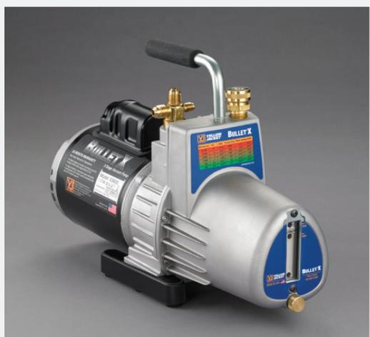
Wide mouth oil reservoir port for easier, cleaner filling. The YELLOW JACKET® BULLET®X vacuum pump is a two-stage rotary vane oil-sealed 7 CFM pump that pulls down to 25 microns or better.
