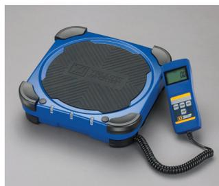
The 220 lb. capacity of the YELLOW JACKET® Digital Charging Scale has a 0.1 oz. resolution and 0.5% accuracy under all conditions. It can be easily re-calibrated in the field with inexpensive reference weights.
