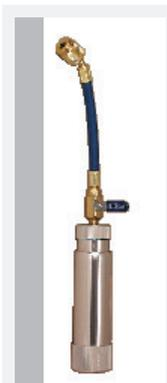
This 2 ounce injector is easy to refill and easy to operate. Calibrations are clearly marked on the injector. Connect to A/C low-side and rotate handle. AC/R and auto models. Maximum port pressure of 250 psi.
