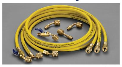
The new A2L refrigerants, R-32 and R-454B, have adopted left-handed connections for their tanks. These new refrigerants are categorized as slightly flammable, so left-handed connections were implemented to differentiate them from A1, non-flammable refrigerants. As the industry adopts these new refrigerants, YELLOW JACKET® A2L Tank Adapters and Charging Hoses incorporate left-handed connections so a service technician can safely charge A2L refrigerant systems.
