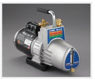
Wide mouth oil reservoir port for easier, cleaner filling. The YELLOW JACKET® BULLET®X vacuum pump is a two-stage rotary vane oil-sealed 7 CFM pump that pulls down to 25 microns or better.
