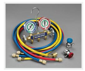
Forged body is solid brass for durability. Full porting maximizes capacity. Metal valve handles are full size for easy operation. Hose anchors are forged into back of body at 45°. Flutterless™ technology helps minimize needle pulsation for easier, more accurate readings. Double "O" ring piston for reliability and long service life.
