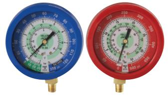
Gauges are completely filled with glycerin for maximum protection from pulsation. Large 3-1/2" (90 mm) diameter gauge with refrigerants color-coded on the dials in bold numbers. Offset stem fits all major manifold brands.
