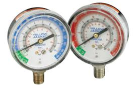
Ammonia gauges are designed for use on manifolds and as permanent gauges on any system or equipment charged with ammonia. The Bourdon tube is made of 316 stainless. The dials show dual temperature and pressure scales. All gauges are equipped with restrictors to protect the gauges against pulsating pressure.
